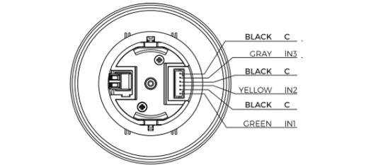
Table mapping inputs to colors: INPUT 1 (DIGITAL) VERDE / GREEN, INPUT 2 (DIGITAL) GIALLO / YELLOW, INPUT 3 (DIGITAL) GRIGIO / GRAY, COM (COM FOR ALL INPUTS) NERO / BLACK.
