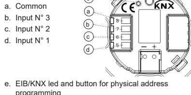
e. EIB/KNX led and button for physical address programming
