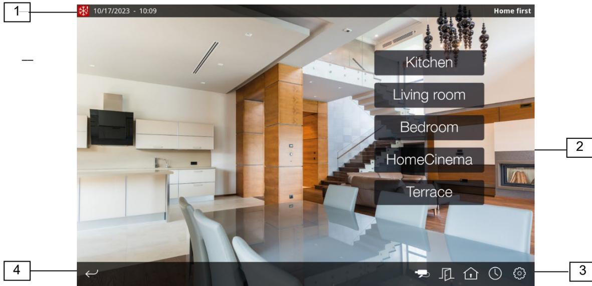
At the top of the screen, the status bar (1) shows the current date and time, as well as the name of the page or function currently shown. This area may also include different icons that provide additional information about the system status.
