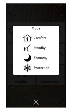
By default, the push button will show the icon and/or text corresponding to the last option that was selected. However, if the Show fixed icon/text parameter is set to "Yes", a fixed icon and/ or text will be displayed on the component instead.
