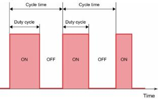
In order to avoid damage to the switching actuator, if the computed on or off time is shorter than 5 seconds, a fixed time of 5 seconds is used instead.
