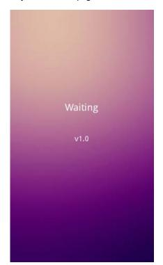
The Synchronisation page will remain onscreen as long as the device has not yet been programmed with application data from ETS. This page is also displayed if the KNX bus is disconnected, or while the device is being reprogrammed.
