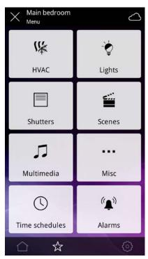
A cloud-shaped icon in the top of the screen ( $\bigcirc$ ) indicates that the connection was established through eTouch.eelectron.cloud. If this icon is not shown, then the connection is direct (LAN). Some of the device functions cannot be accessed from the app,
