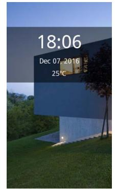
Upon startup, the Home page is shown automatically. The Home page can be configured to show the current date and time, and also the current temperature. Tapping anywhere on the screen will automatically switch to the "default page". The "default page" can be the Menu page, the Favorites page, or any of the configured control pages.
