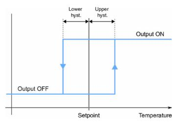
Two-point control with hysteresis is easy to setup and can be used with regular switching actuators. However, it is also sub-optimal in terms of power consumption and comfort, due to the typical fluctuations of the room temperature around the setpoint which arise as a result of the simple control algorithm.
