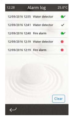
An internal alarm log holds information about the latest 100 alarm events, including the event date and time. The alarm log can be reached from the alarms page ("Alarm log") button. The following events are logged:
