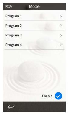
The "Enable" checkbox allows to manually enable or disable any configured actions. Note that this checkbox will be disabled if the component belongs to a timer group that is currently locked. Selecting a program shows the program edit page, where all the parameters for the timer program can be edited.
