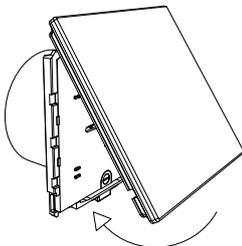
4. To remove the cover, push the pin on the bottom of the plastic cover, then remove first the bottom and then the top.
