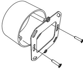
2. Connect the KNX cable to the device and fix it to the metal frame with the appropriate screws included.
