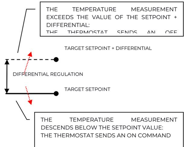
The following image instead shows the operation of the on/off control in cooling.
