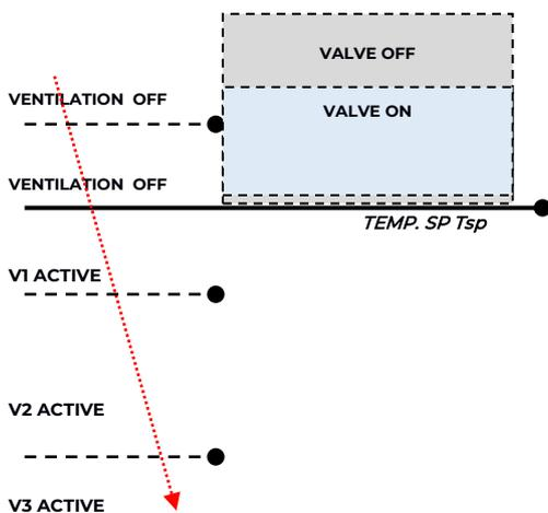
If parameter "Fancoil valve" in the "Thermostat Settings" page is set to "proportional", valves are set as independent and parameters "bandgap" and "proportional band [Bp]" can be set specifically for both cool and heat status.
