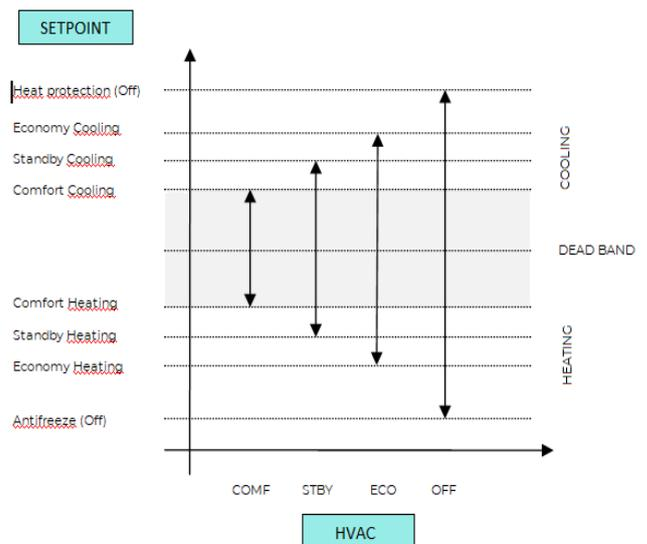
The following image clarifies the concept. It is possible to set the comfort setpoint as the centre of the dead band through the relative parameter; the comfort value is common to the heating and cooling modes.
