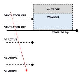
If parameter "Fancoil valve" in the "Thermostat Settings" page is set to "proportional", valves are set as independent and parameters "bandgap" and "proportional band [Bp]" can be set specifically for both cool and heat status.
