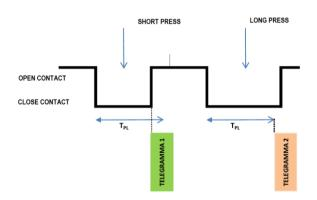
When the input is closed, the time count starts; if the input is opened before the time exceeds the time  $T_{PL}$ , the device executes the command
