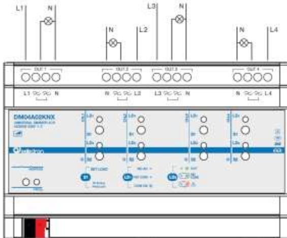
Connection diagram for output combined
