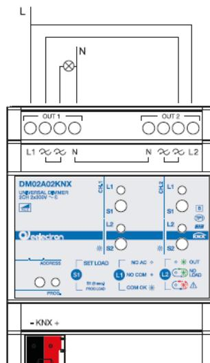
**⚠** The 2 channels can work with different LINES (PHASE) ; it is necessary to correctly identify the NEUTRAL since it is the same for both channels and is internally connected between the 2 output channels!
