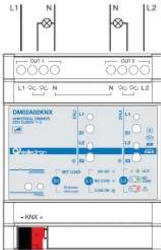
Connection diagram for output combined
