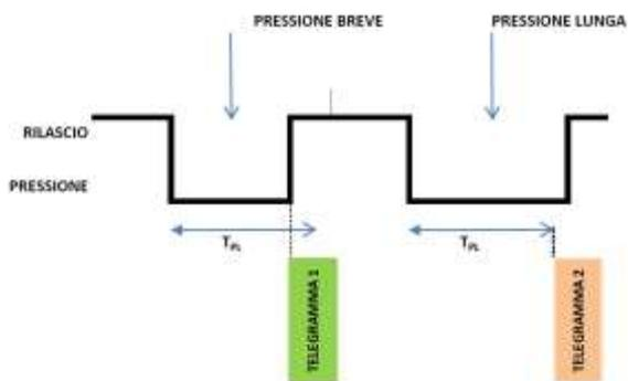
When button is pressed then counting time starts; if the button is released before time exceeds TPL time, device executes the command associated with the event of "short press" and if, on the contrary, TPL timeout expires and button is still pressed then the command associated with the event of "long press" is executed.
