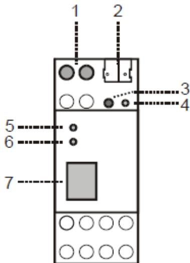
1: Connector for external power supply (12 V to 24 V AC/DC)
