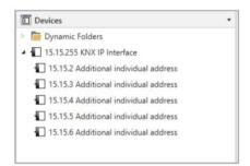
Each individual KNX address can be changed by clicking on the list entry and typing in the desired address into the "Individual Address" text-field. If the text-field frame switches to color red after entering the address, the address is already taken within your ETS project.
