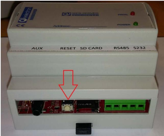
Press the RESET-button until the SERVICE-LED starts blinking (minimum 10 seconds). Then release the RESET button.
