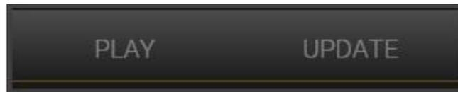
By clicking the PLAY button, the value configured for the parameter “VALUE KNX SCENARIO” will be sent to the KNX bus and the KNX devices configured for the usage of the KNX scenario will start the actions memorized for the received number.
