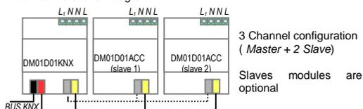
Dimmer DM01D01KNX can be used in one of the following configurations:
