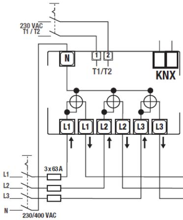
**Neutral wire must be connected to the meter**
