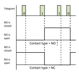
Behavior of the relay set to "NO" and "NC" when activation telegram is telegram "0":
