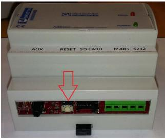
Press the RESET-button until the SERVICE-LED starts blinking (minimum 10 seconds). Then release the RESET button.
