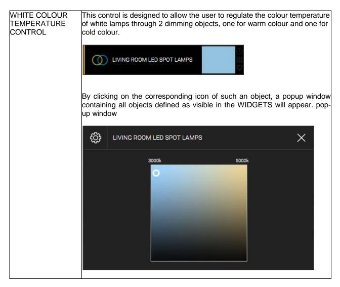
Besides the 2 objects for the dimmer control it is also possible to connect other 2 objects (typically virtual objects, check out the corresponding chapter in this manual) in order to label the maximum and minimum temperature; in this case you can just insert the values in the "LABEL" column of the administration page of the complex object:
