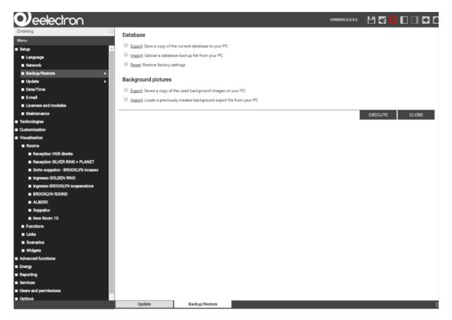
After the desired action has been selected (and in case of the import action a suitable backup has been selected), click on "EXECUTE" and wait for the desired action to be processed.
