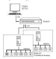
The KNX IP Router has a filter table and is able to buffer up to 150 telegrams.
