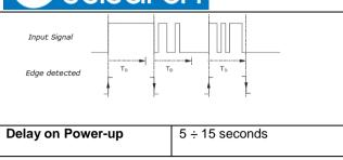
Through this parameter is possible to set the delay of transmission of telegrams after a power on by selecting the time by which the device is allowed to send telegrams.
