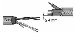
5. Do not damage the electrical continuity conductor of the shielding.
